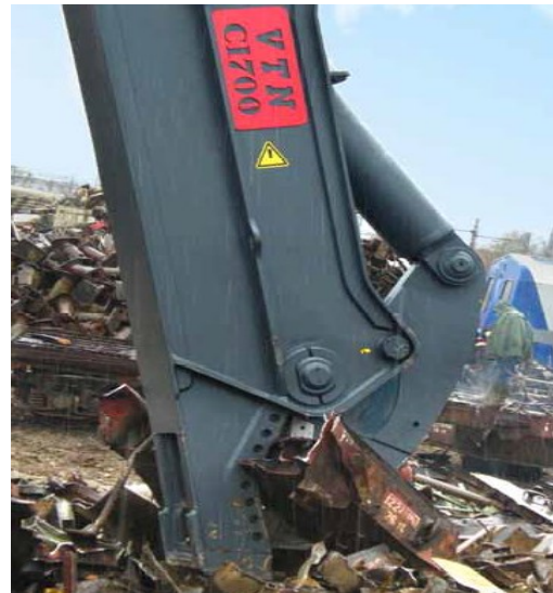
CI Iron & Steel Shear with changable and reversible shear og integrated 360° rotation
