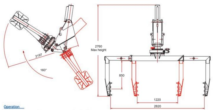
Model UHL2705 requires three seperate services at the jib, with respective operating levers at the crane base. This model achieves all motions, ie. tilt, clamp and rotate totally independent of the actual crane operation.
