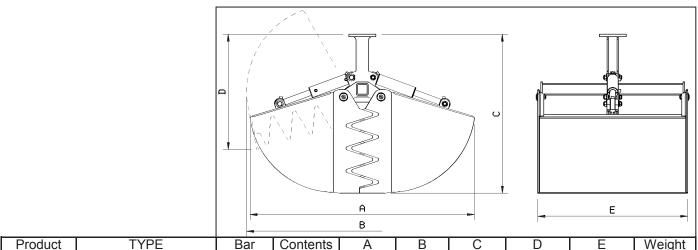
Ε Weight mm mm mm mm kg mm no. SP 2 CV 50-80 1000 470 3030 5420 200 1000 L 1690 1770 1175 1260 750 3030 5440 SP 2 CV 50-80 1500 200 1500 L 1920 1980 980 1280 520 1360
