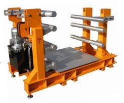
**HEMA Clamp Device** is intended for handling refrigerators and other appliances, televisions and similar products that are to be disposed of as paper and paper balls.
